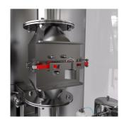
Safety system to avoid contamination from metal parts and damage to machinery removing extraneous matters from equipment installed downstream. Magnets are covered with a detachable pipe and do not come into contact with the product. Easy to clean and suitable for all powders.
