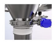
Extraction and locking machine that ensures leak-tightness up to a 1.5 bar. No leaks and no loss on loading. Suitable for all powders and abrasive products thanks to the gasket in long-lasting anti-abrasive rubber. Body in cast iron, disk in stainless steel, inductive limit switch, double acting pneumatic actuator and inductive limit switch. Operating temperature up to 100°c.
