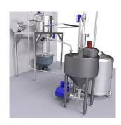
Centralized systems for the production, storing and metering of salt solution. Ideal when a cold dough is needed (below zero) to prevent eccessive heating during processes such as fermentation, avoiding the problem of water freezing. Salt solution also makes it easier to to amalgamate the salt in the dough.
