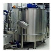
Metering of fat products in liquid form, in stainless steel tanks with heating system, optimized circulation and fat cutting knife on multiple levels.
