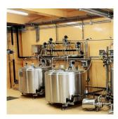
Cleaning system for a complete hygienization of tanks and pipes, particularly recommended for processes including oil, eggs, and yeast. Manual or automated washing, detersion, recircle and recovering processes through an integrated management of pumps and valves on the pipes.
